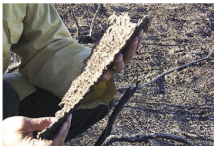
Plate 14 Hydro-mulching forming a protective soil layer (USDA 2006)
