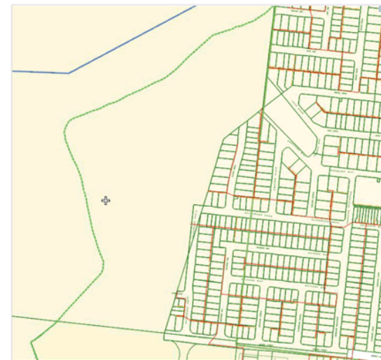
Fig 13. Existing local sewer network
