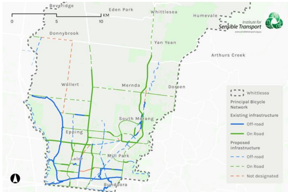
Figure 13: Principal Bike Network – Existing and proposed infrastructure (Background Paper, Institute for Sensible Transport, 2023)
