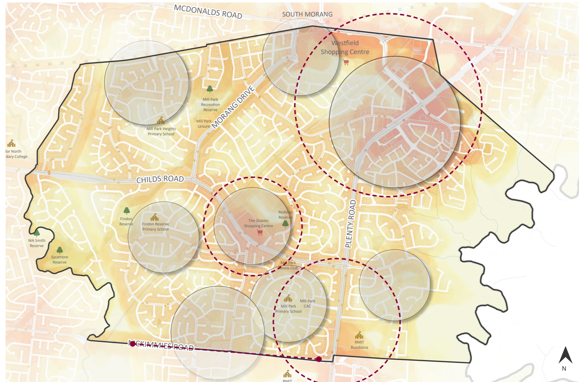
Figure 59 Base map shows combined heat map of walkability to open spaces, PTV and town centres and opportunities to increase density.
