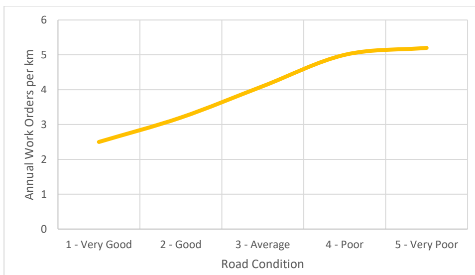
Figure 8.1 – Work Orders by Condition per Kilometre of Road (2021)
