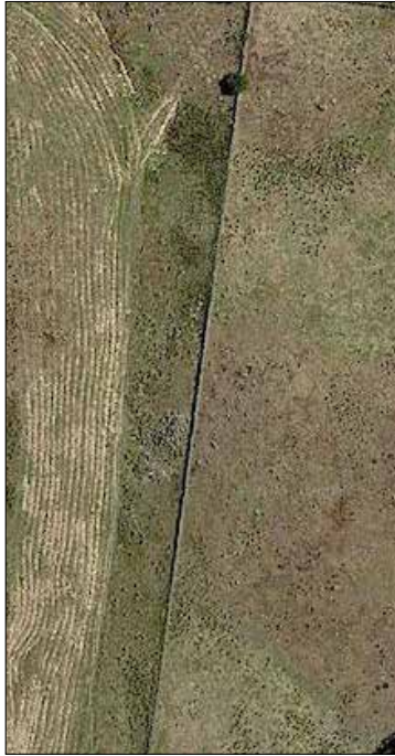
Images 53, 54: Walls over stony rises. These views clearly show the contrast between the high and intact structure of walls as they pass over stony rises, and their breakdown over softer ground. The wall at left is an original north-south boundary wall on the Medland Estate, east of Bodycoats Road. The wall at right is the east-west boundary wall between 240 & 270 Bindts Road. (Google satellite, 2019)
