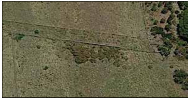
Images 53, 54: Walls over stony rises. These views clearly show the contrast between the high and intact structure of walls as they pass over stony rises, and their breakdown over softer ground. The wall at left is an original north-south boundary wall on the Medland Estate, east of Bodycoats Road. The wall at right is the east-west boundary wall between 240 & 270 Bindts Road. (Google satellite, 2019)
