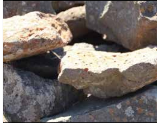
Image 115: On stony rise near the cemetery, weathered by expanding and contracting moisture in a crack of the volcanic stone, a surface of the rock has broken away naturally (left); these concave stones (right) were often picked up (or easily knocked off the rock) and became 'coverbands' to bed the copings. (David Moloney, 2019)
