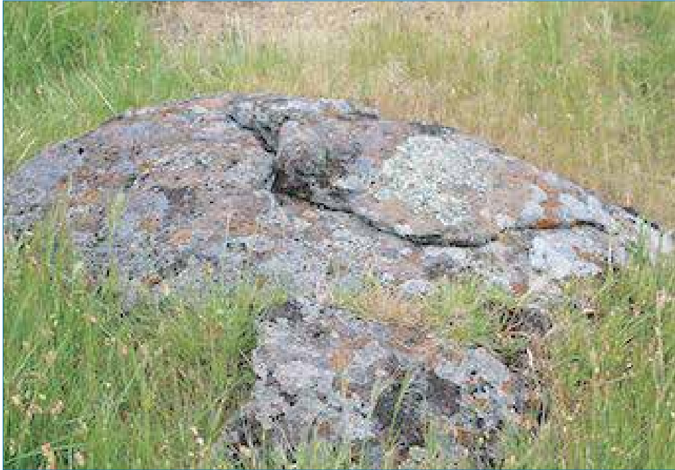
Image 6: O'Hern's Road near Merri Creek: surface stone on top of stony rise, showing natural horizontal fracture. This example may be too slim for building, but this style of flat-bottom stone could easily be prised off with a crowbar, or tapped off with a heavy hammer. (David Moloney, 2019)
