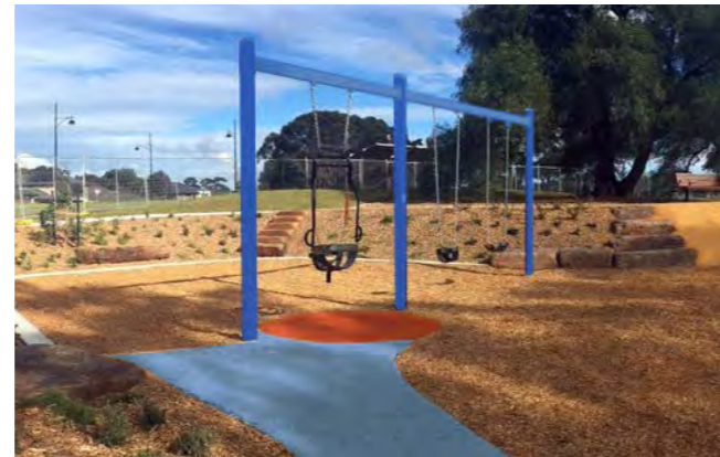
1.5 Three bay steel swing with toddler seat, standard seat and all abilities seat
