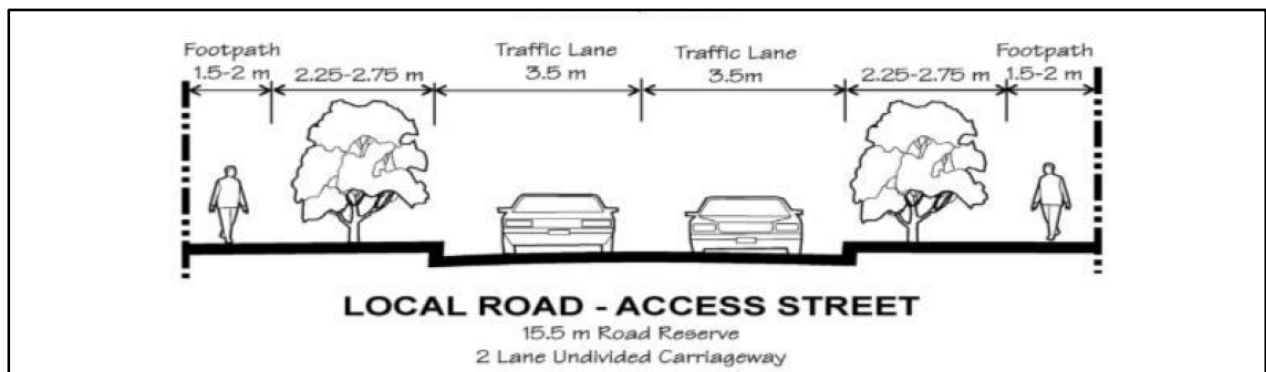
Figure 24 Local Access Street (15.5m) – Applicable to internal roads within the development area
