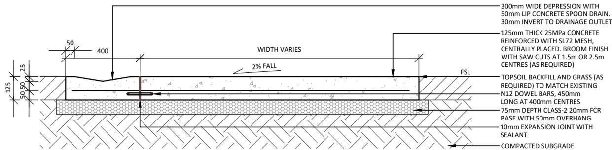
01 CONCRETE PATH AND SPOON DRAIN - SECTION
