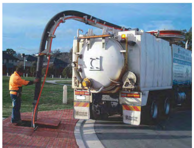
Figure 53 Service vehicle reach for gross pollutant traps
